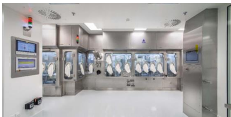
Figure 2 Filling line with isolator for larger volume containers (courtesy of SKAN AG)
